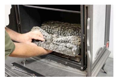
6. Lift the burner out of the firebox. Lift the front edge first then pull it up and out of the firebox. Natural gas stoves will have a narrow air shield attached to the burner.
