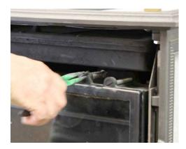
3. Use a 7/16" socket or wrench to remove the glass retainer at the bottom front of the firebox. (NOTE: For each bolt, there are 2 spacer washers in between the retainer and the front casting. Be careful not to lose them!)
