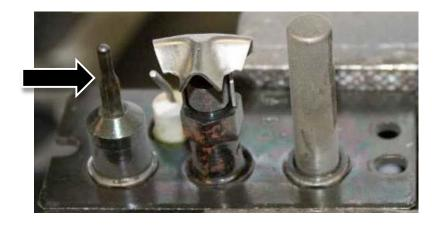
8. Remove the screws that hold the pilot assembly in place, and gently lift the assembly up. Lift it high enough to cut the copper lead to the thermocouple. **Do not cut any other lines to the pilot assembly.**
